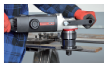
Steel plate beveling
